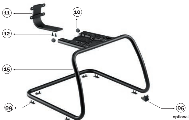
15 sl46-base a slitta in tubo 25 tappi esclusi sl46-slide frame pipe ø25 without caps
