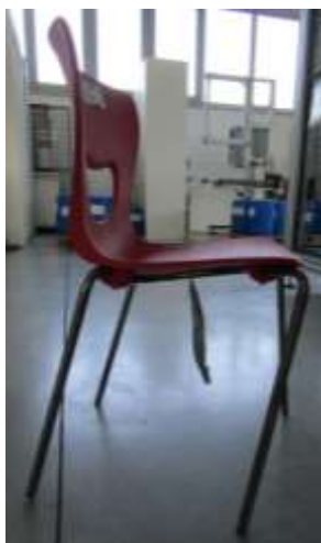
Detail of permanent deformation after test on one front leg
