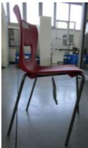
Detail of permanent deformation after test on one front leg
